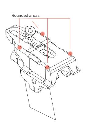
sired. At your selected saddle angle, make sure the carrier bolts engage all threads of the threadinserts and stick out between 1 and 5 mm, using the different length supplied bolts. If the bolts stick out too far, either cut them to the correct length or jump to step \*2. Install the saddle\*, and check whether the saddle at full load (e.g. jumping up from the saddle and dropping your full weight onto it) collides with the bolts sticking out. If it does, shorten the bolts.
