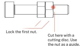
full weight onto it) collides with the bolts sticking out. If it does, shorten the bolts.
